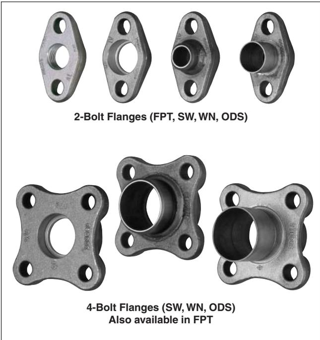
Flanges for sizes 5-25mm (3/16" to 1") are a 2-bolt oval style. Flanges for sizes 32-100mm (1 1/4" - 4") are a 4-bolt square style. Flanges for sizes 125-150mm (5" - 6") are an 8-bolt round style and are available as male type only.
