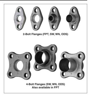
Flanges for sizes 5-25mm ( $\frac{3}{16}$ " to 1") are a 2-bolt oval style. Flanges for sizes 32-100mm ( $\frac{1}{4}$ " - 4") are a 4-bolt square style. Flanges for sizes 125-150mm ( $\frac{5}{16}$ " - 6") are an 8-bolt round style and are available as male type only.
